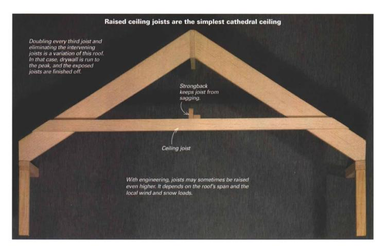
roof were changed to a cathedral style, I'd use at least 2x10 rafters. The reason is twofold. Extra heft helps to keep the rafters from sagging over time. And without flat ceiling joists, the insulation goes in the roof. The rafters must be wide enough to accommodate the insulation plus space for ventilation.
