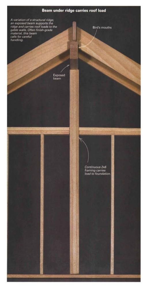
they butt to the inside of the gable rafters. Even after deducting  $1\frac{1}{2}$  in. for the gable rafter, the beam has a full 4 in. of bearing. I stagger these shorter members down so that they're about  $\frac{1}{2}$  in. lower than the top of the rafters. This method allows air to flow to the ridge vent. After nailing the beam together, I measure, cut and then install the post under the beam to carry the load downward.
